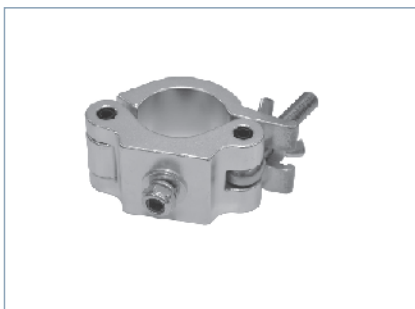
ACS-TC50-30 For tube diameter 48-51mm, clamp width 30mm, load capacity 200kg.
