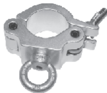
ACS-TC50-502S For tube diameter 48-51mm, clamp width 50mm, load capacity 250kg.
