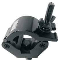
ACS-TC30-50B For tube diameter 48-51mm, clamp width 30mm, load capacity 250kg.
