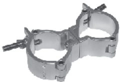
ACS-TC50-502D For tube diameter 48-51mm, clamp width 50mm, load capacity 100kg.
