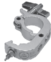
ACS-50-30S For tube diameter 48-51mm, clamp width 30mm, load capacity 250kg.
