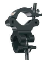
ACS-TC50-50B For tube diameter 48-51mm, clamp width 50mm, load capacity 500kg.
