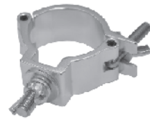
ACS-TC50-50S For tube diameter 48-51mm, clamp width 50mm, load capacity 100kg.
